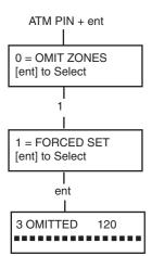
When enabled, the **Forced Set** option allows the user to automatically omit zones, eligible for omission, which are open when the system setting routine is started. Zones omitted in this way remain omitted for one set period only.
